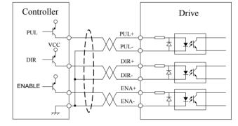
Figure 3: Connections to open-collector signal (common-anode)
