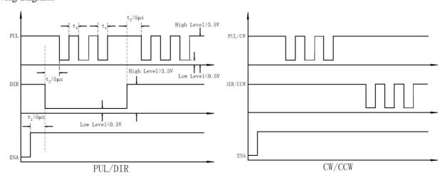
Figure 11: Sequence chart of control signals
