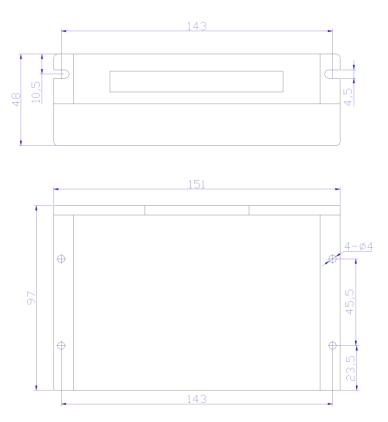
Figure 1: Mechanical specifications
