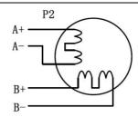
Figure 5: 4-lead Motor Connections
