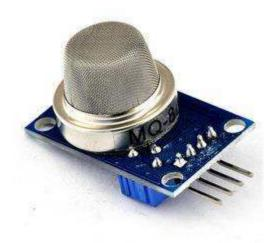
This sensor module has an MQ-8 as the sensor component and has a protection resistor and an adjustable resistor on-board. The MQ-8 gas sensor is highly sensitive hydrogen and less sensitive to alcohol, and cooking fume. It could be used in gas leakage detection appliance in family and industry. The resistance of the sensor component changes as the concentration of the target gas changes.
