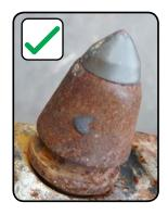
The teeth need to rotate while drilling to maintain an efficient cutting tip. The tungsten tip and tooth should be evenly pointed.
