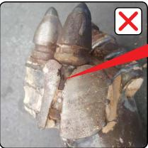
Failure to change worn teeth will cause damage to the auger body and pilot requiring a new pilot or a costly repair. Always ensure the pilot teeth are rotating and in perfect condition.
