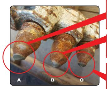
Teeth that look like **A** have not been rotating in the pocket and as a result the tooth is uneven and will cut poorly. We recommend changing this tooth.
