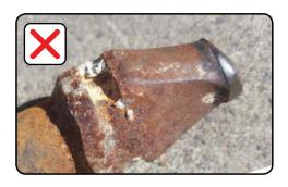
Flat spots indicate that teeth are not rotating freely in their pockets when drilling. The tungsten tip has lost its point and no longer offers the best cutting efficiency. If this occurs, replace the tooth immediately.
