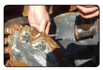
Use a punch or a rotating pick removal tool to remove teeth.
