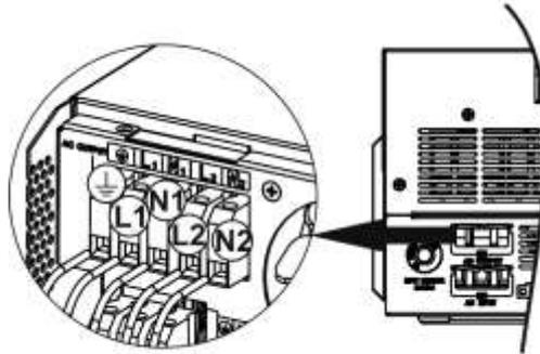
5. Make sure the wires are securely connected.
