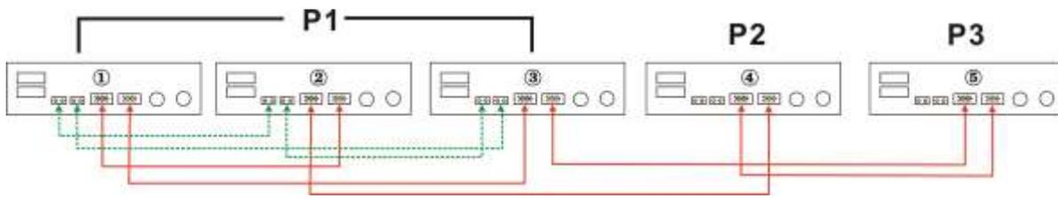
Two inverters in two phases and only one inverter for the remaining phase:
