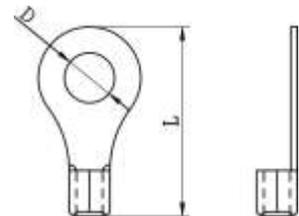
**Recommended battery cable and terminal size:**
