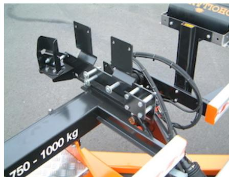
OAM014 - Quick-fit mounting plates per type of vehicle
