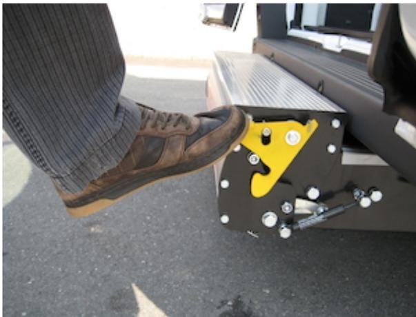
Unlocking by foot upon platform deployment. Automatic locking upon stowage
