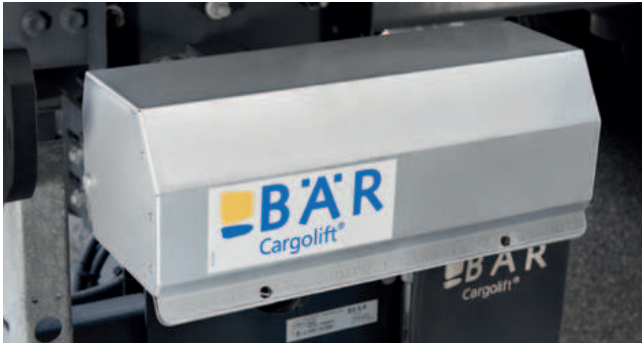
Protection cover (option) for Bär Control EVO made of stainless steel.
