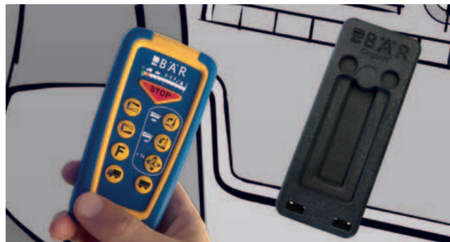
Bär SmartControl Plus with docking station (option) with rechargeable hand-held transmitter (instead of battery-powered transmitter). Cabin switch via radio and starter interruption possible.
