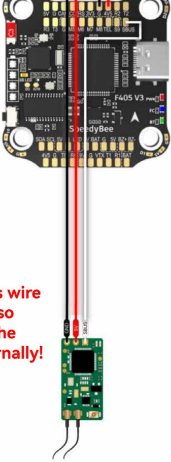
Disconnect this wire because it is also connected to the SBUS pad internally!
