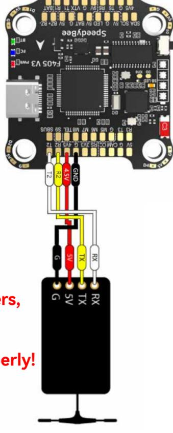
For some ELRS receivers, it is necessary to disconnect this wire in order to function properly!
