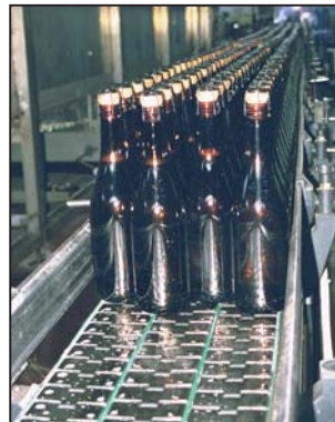
uni SS 881 TAB-K325 Side flexing Beer bottles 3 track Lubricant: Soapy water
