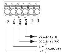
Connectors ST+ / ST- are only used for sensor types which additionally have a passive resistance sensor element for temperature measurement.
