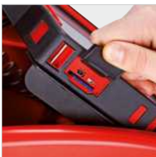
Cover protected connections for SD card, Micro-HDMI and Mini-USB
