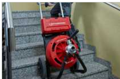
Easy transport due to stair capable chassis
