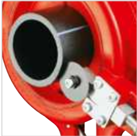
ROCUT 110 with cutter wheel (No. 54950) (special accessories)
