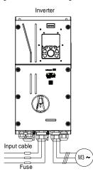
Figure 4-19 Fuse configuration
