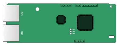
The terminal CN2 adopts standard dual RJ45 interfaces, and the two RJ45 interfaces are not distinguished from each other and can be interchangeably inserted.
