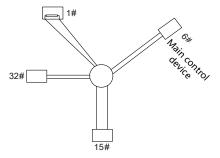
Use shielded cable, if possible, in multi-device connection. The baud rates, data bit check settings, and other basic parameters of all the devices on the RS485 line must be set consistently, and addresses cannot be repeated.
