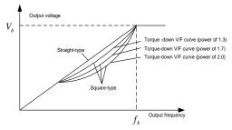
The S1 IP55 series Inverter also provides multi-point V/F curve. Users can alter the V/F curve outputted by Inverter through setting the voltage and frequency of the three points in the middle. The whole curve consists of five points starting from (0Hz, 0V) and ending in (fundamental motor frequency, rated motor voltage). During setup, it is required that  $0\le 1\le 2\le 3\le 1$  and  $0\le 1\le 2\le 3\le 3$ .
