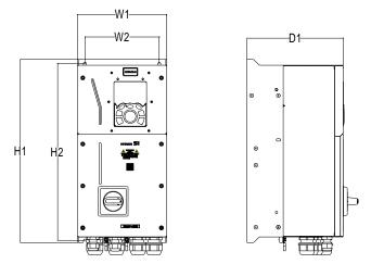
Figure C-2 Wall-mounting diagram of Inverters of 4.0–37kW
