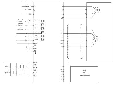
The following figure shows the external wiring of the EC-PG504-00 expansion card.
