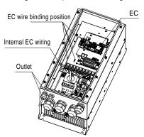
Figure A-4 Expansion card wiring
