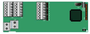
SW1 is the start/stop switch of the programmable expansion card. CN1 contains terminals PE, 485-, 485+, GND, Al1, and AO1, and a selection jumper resides on the next. "Al" and "AV" are the current type input selection and voltage type input selection of Al1, and they can be
