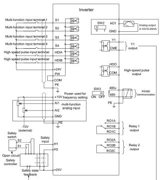
Figure 4-15 Wiring diagram of control circuit
