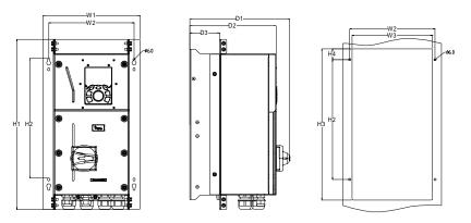
Figure C-4 Flange mounting diagram of Inverters of 4.0–37kW
