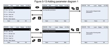
After selecting a specific function code, press 😎 key to enter the parameter addition
