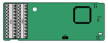
The dual in-line package (DIP) switch SW1 is used to set the voltage class (5 V or 12 V) of the power supply of the encoder. The DIP switch can be operated with an auxiliary tool.
