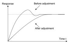
**Stabilize the feedback value as fast as possible:** when overmodulation occurred, shorten integral time (Ti) and prolong derivative time (Td) to stabilize control as fast as possible.
