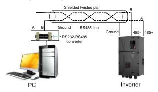
Figure 9-1 Wiring of RS485 applied to one Inverter
