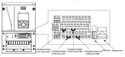
Figure 4-16 Position of U-shaped jumper
