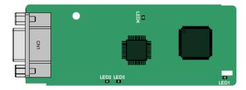
CN1 is a 9-pin D-type connector, as shown in the following figure.
