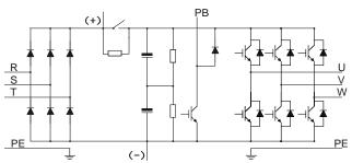
Figure 3-1 400V (4kW-15kW) main circuit diagram
