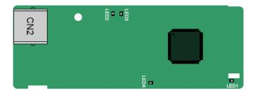
The EC-TX504 communication card adopts standard RJ45 terminals. The EC-TX504 card supports S1 DriveManager software. For usage with standard Ethernet/IP protocol, please install the EC-TX510 card.
