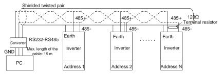
Figure 9-5 shows the start connection diagram. When this connection mode is adopted, the two devices that are farthest away from each other on the line must be connected with a terminal resistor (in Figure 9-5, the two devices are devices 1# and 15#).
