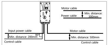
Figure D-4 Cable arrangement distance
