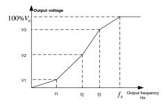
The S1 IP55 series Inverter provides dedicated function codes for V/F control mode. Users can improve the performance of V/F through settings.
