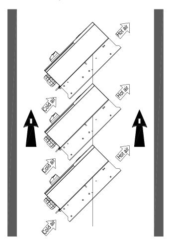
Figure 4-6 Tilted installation
