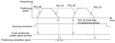
P21.25 Hold time of positioning completion signal
