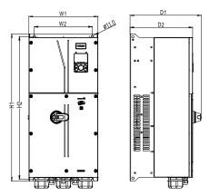
Table C-2 Wall-mounting dimensions of Inverters (unit: mm)
