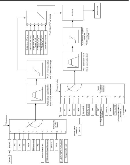
When selecting customized V/F curve function, users can set the reference channels and acceleration/deceleration time of voltage and frequency respectively, which will form a real-time V/F curve through combination.
