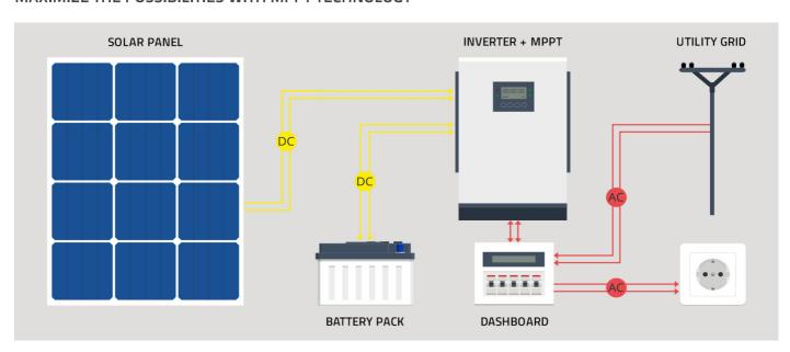
The battery charging inverter uses a state-of-the-art 100A MPPT charge controller to maximize the power drawn from the photovoltaic panels, using advanced maximum power point tracking technology.
