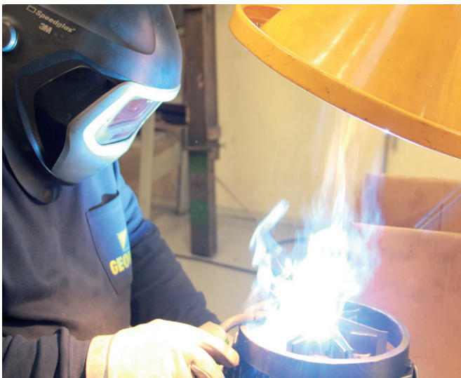
COMPACT arm 1-2m installed and including automatic control devices for automatic start/stop of the fan and motor damper.
