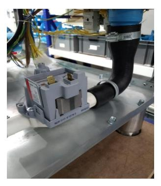
As you can see from the picture, the Drain Pump should be connected to the black hose and with the help of hose clamp, the left side of the hose (black hose) should be tied properly to the drain pump.
