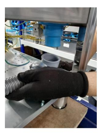
This is the hose for Hood Type Dishwasher without Drain Pump. So, if you want to replace it with Drain Pump, you should remove the gray hose first.
