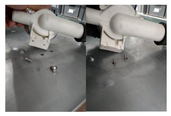
The drain pump must be affixed to the body from the bottom side with the help of screws as shown in the picture.
