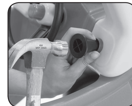
Place axle cap tool over ignition base and hammer.
