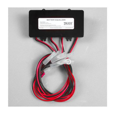
BE48 battery equalizer is energy transfer type equalizer, it can compensate for batteries with two sides. The equalizer starts to work when there are 10mV between two batteries. The current will flow from a higher voltage to low voltage, eventually reach equilibrium. It can connect with batteriy system with 24 hours, to keep the system energy balance automatically, no need manual maintenance.
