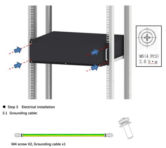
The grounding cable end with screw press-fit fixation in the chassis rear grounding hole, the other end is connected to the frame ( or cabinet ) grounding copper bar to ensure the stable connection.
