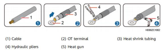
• When installing the power cable, ensure that the protruding part of the OT terminal on the cable must be facing outward.
