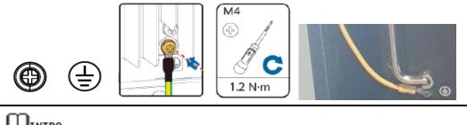
Lt is recommended that silica gel or paint be used around the ground terminal after the PE cable is connected.
