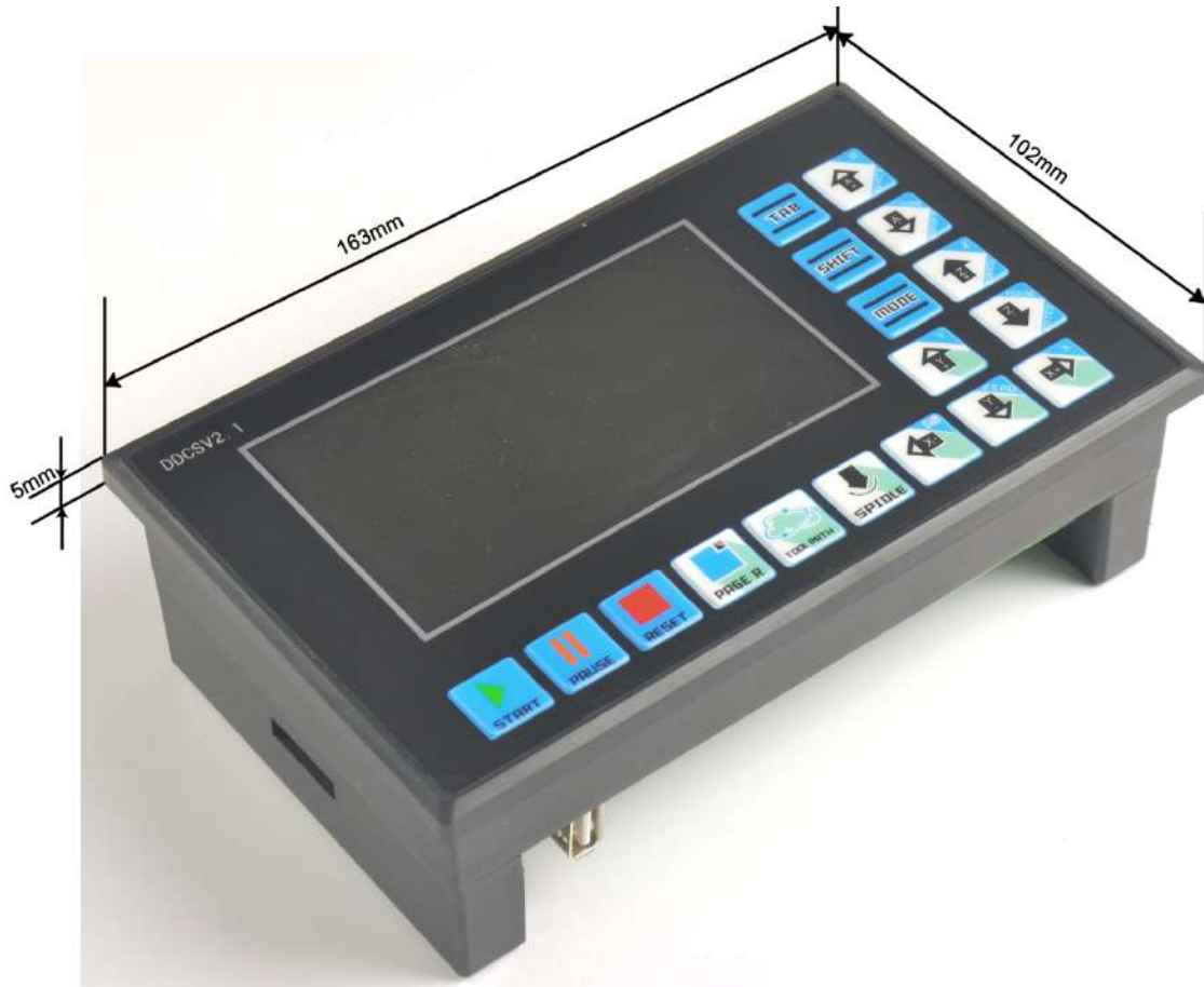
Picture1-1 DDCSV2.1Front external view and dimension figure
