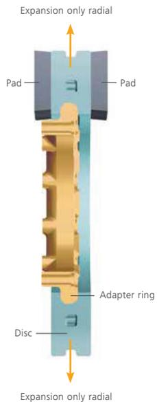
The INTEGRAL disc is cast onto a splined adapter ring and bolted to the wheel hub. The connection between the adapter ring and the brake disc has absolutely no play – without the two parts being fused together. This is the advantage: By composite casting of disc and adapter, the disc can expand radially and contract again during cooling down.
