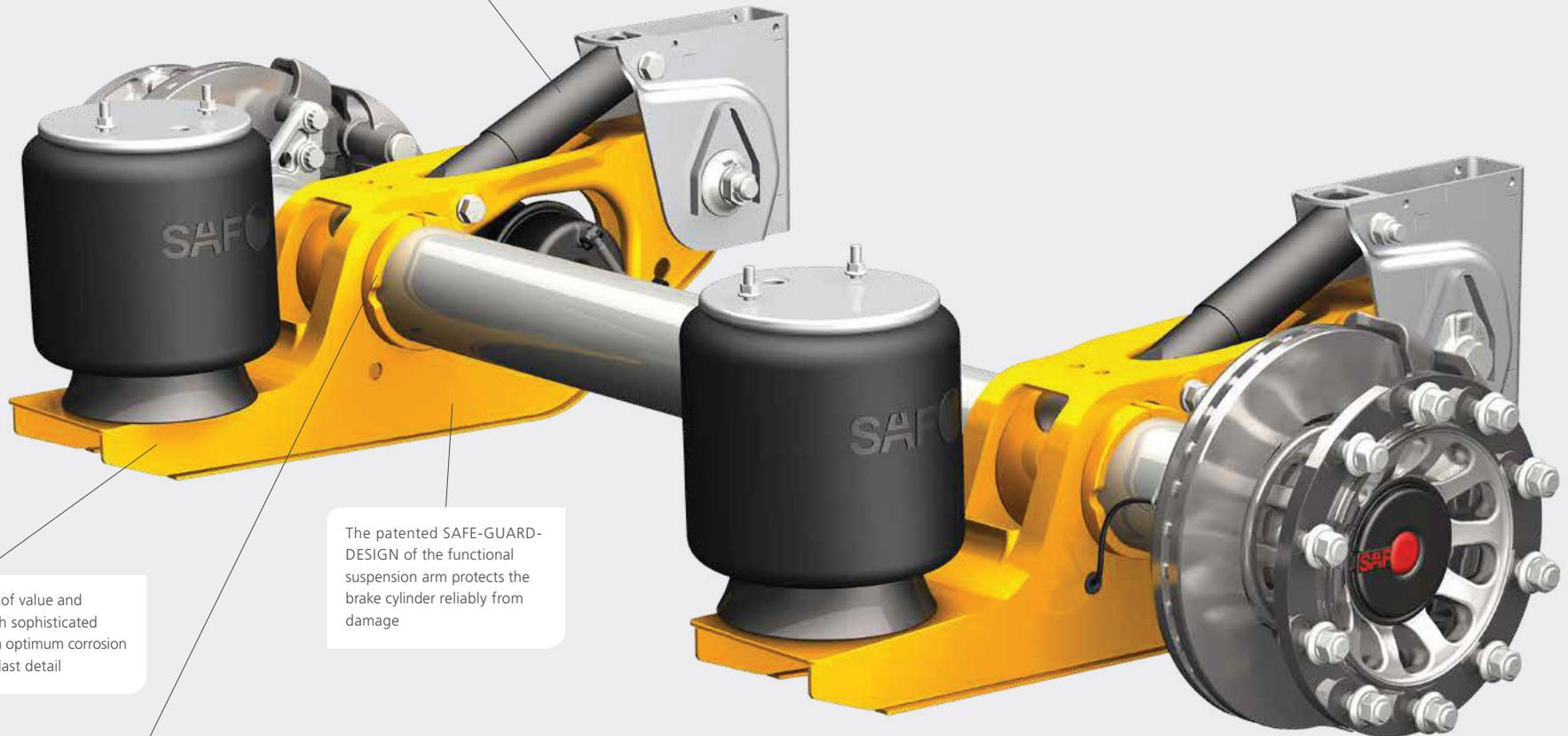
Long-term conservation of value and functional safety through sophisticated cathodic dip coating with optimum corrosion protection down to the last detail
