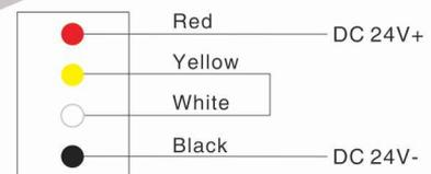
MINI Magnetic Lock with Signal Output
