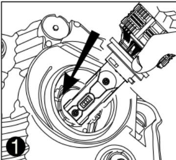
Insert the lamp body as the direction of arrow
