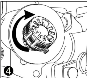
Fix the lamp body by rotate
