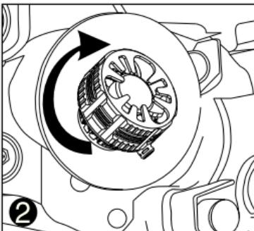
Fix the lamp body by rotate 45° clockwise
