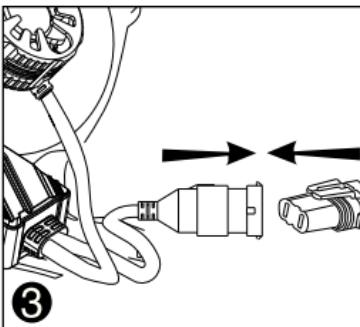
Connect the power line with original car lamp connector
