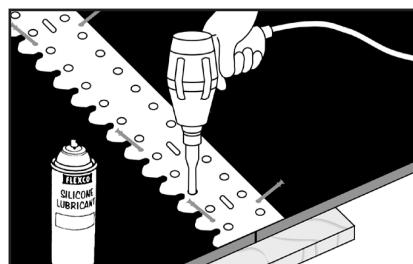
**NOTE:** A  $\frac{1}{2}$ " square drive electric impact wrench with Flexco 5552 Quick Change Chuck will speed hole boring operation. Max torque: 250 Lb-Ft (340 N-m).
