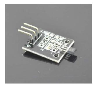
Analog magnetic sensor module and a digital interface, built-in 13 LED build a simple circuit to produce a magnetic flash
