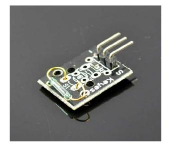
Reed module and the interface comes with digital 13 LED build a simple circuit to produce a Reed warning lamp
