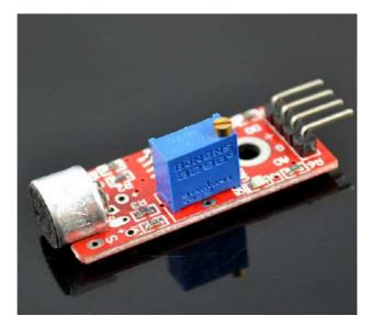
For sound detection Module has two outputs: 1, AO, analog output, real-time output voltage signal of the microphone
