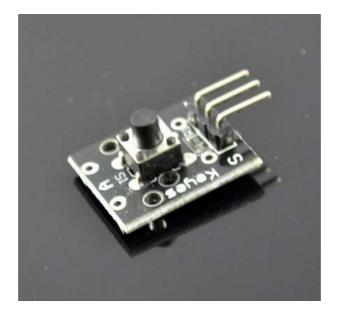
Key switch module and a digital interface, built-in 13 LED build a simple circuit to produce key warning lamp 13 comes with digital interfaces of the LED, the access number 3 button switch sensor interfaces, when the key switch Sensor senses a key signal, LED lights, otherwise off. Routines source code: int Led = 13 ;// define LED Interface int buttonpin = 3 // define the key switch sensor interface ; Int val ;// define numeric variables val void setup () {
