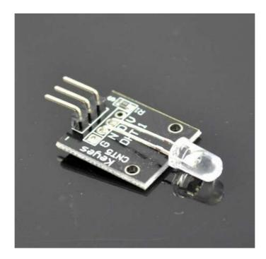
7 color flashing LED module automatically uses 5mm round high-brightness light-emitting diode which has the following characteristics:
