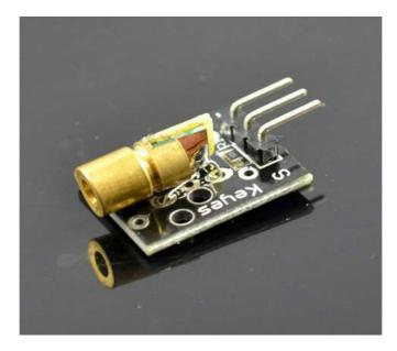
13 laser transmitter module and a digital interface, built-in LED build a simple circuit as shown below
