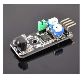
Infrared obstacle avoidance sensor is designed for the design of a wheeled robot obstacle avoidance sensor distance adjustable. This ambient light sensor
