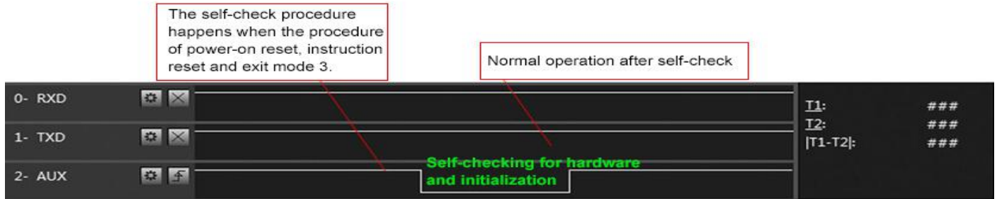
Timing Sequence Diagram of AUX when self-check
