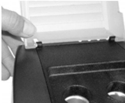
Figure 4 Changing the Protective lid (Step 1)
