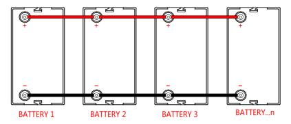
The voltage difference between each battery pack is ≤100mv;
