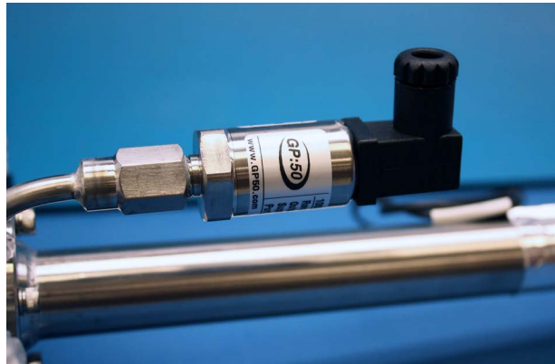
Figure B-9 Newly installed pressure sensor positioning
