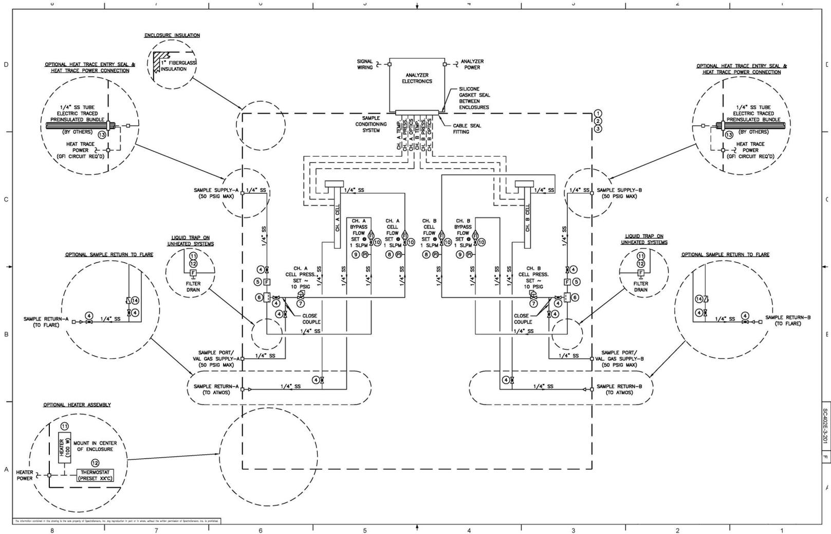
Figure A-8 SS3000e dual stream analyzer system sample system schematic (sheet 1 of 2)
