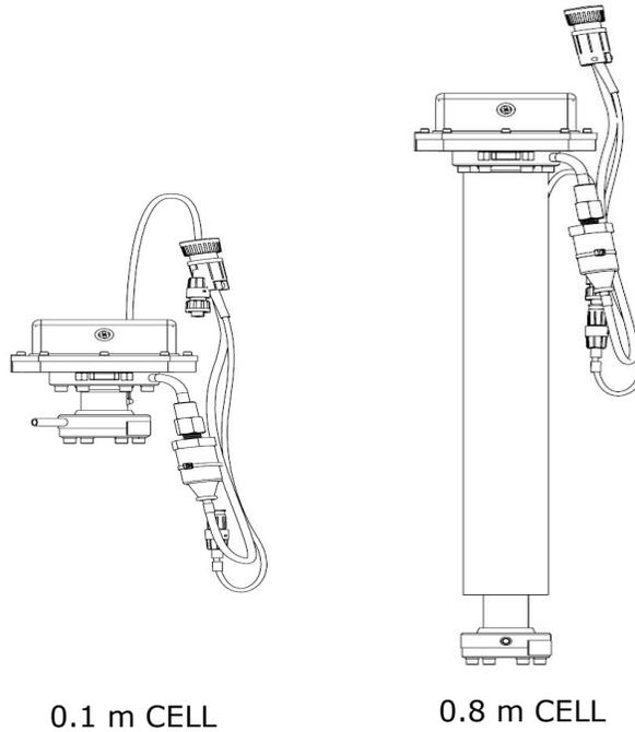
**Figure B-1** Measurement cell types
