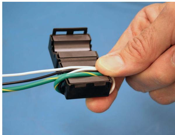
6. Make sure the ferrite ends up as close to the entry point of the wires as possible, as shown below.
