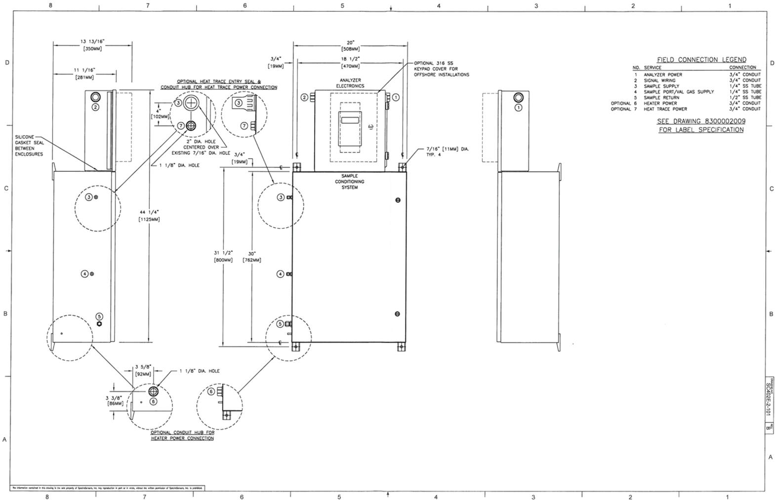
**Figure A-4** SS3000e single stream analyzer system outline and mounting dimensions
