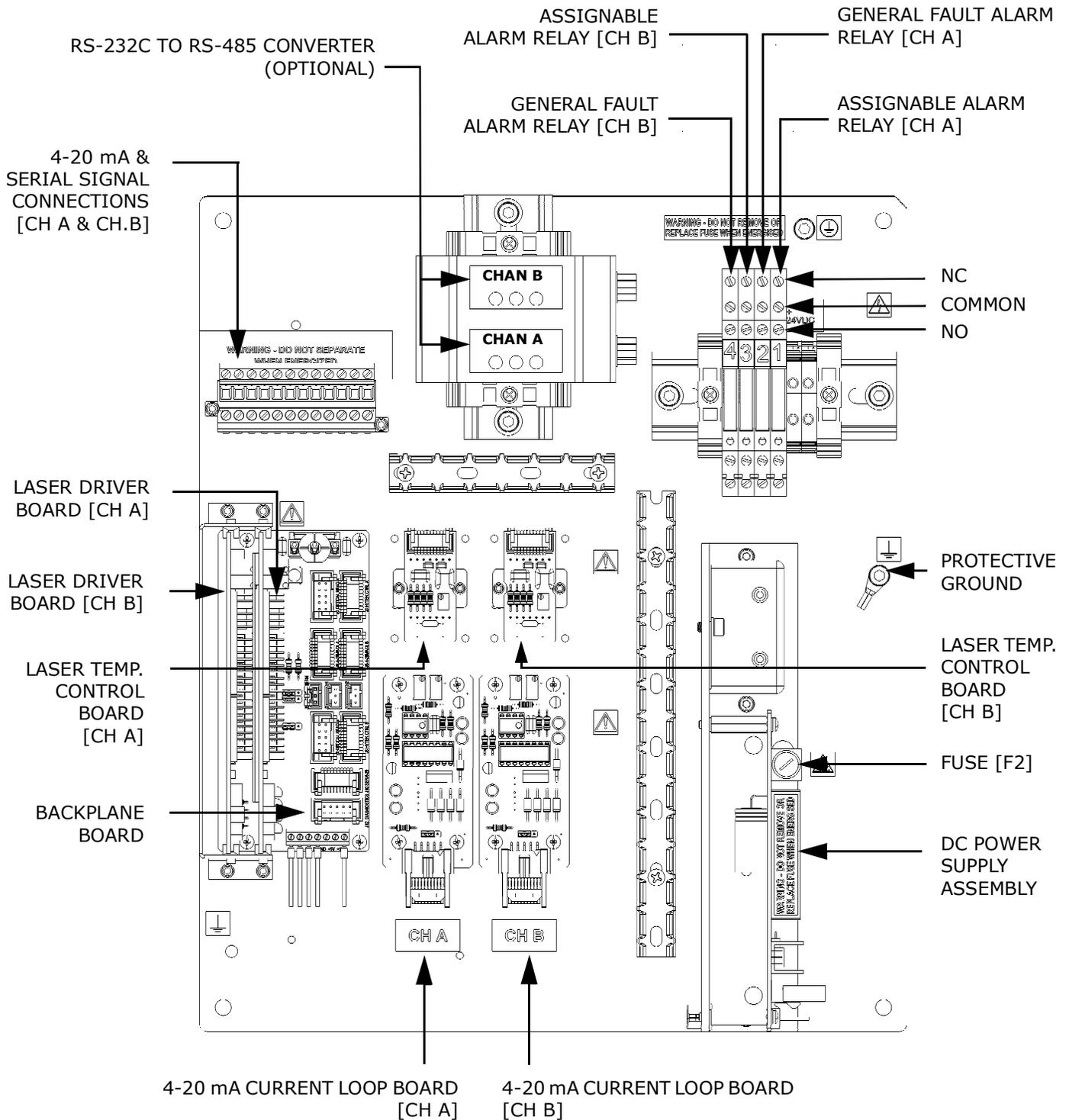
**Figure 1-9** Electronics control board (DC) for dual-channel systems (SS3000e) with RS-232C to RS-485 converter
