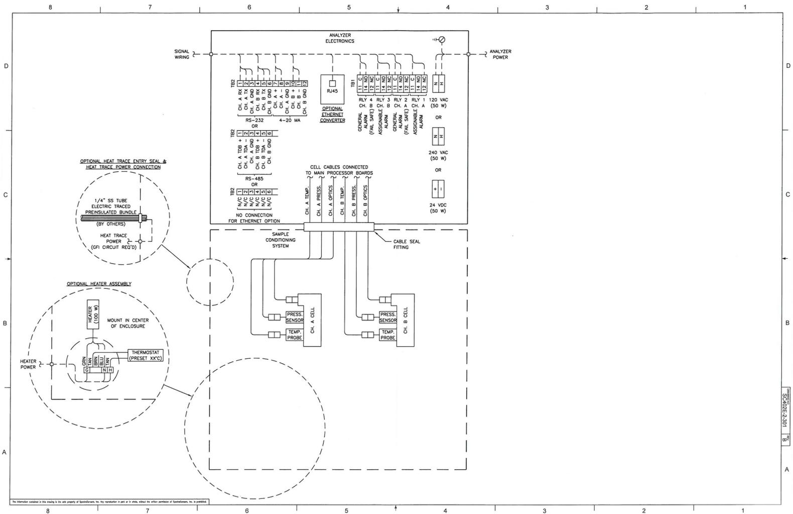
Figure A-6 SS3000e single stream analyzer system power and signal wiring
