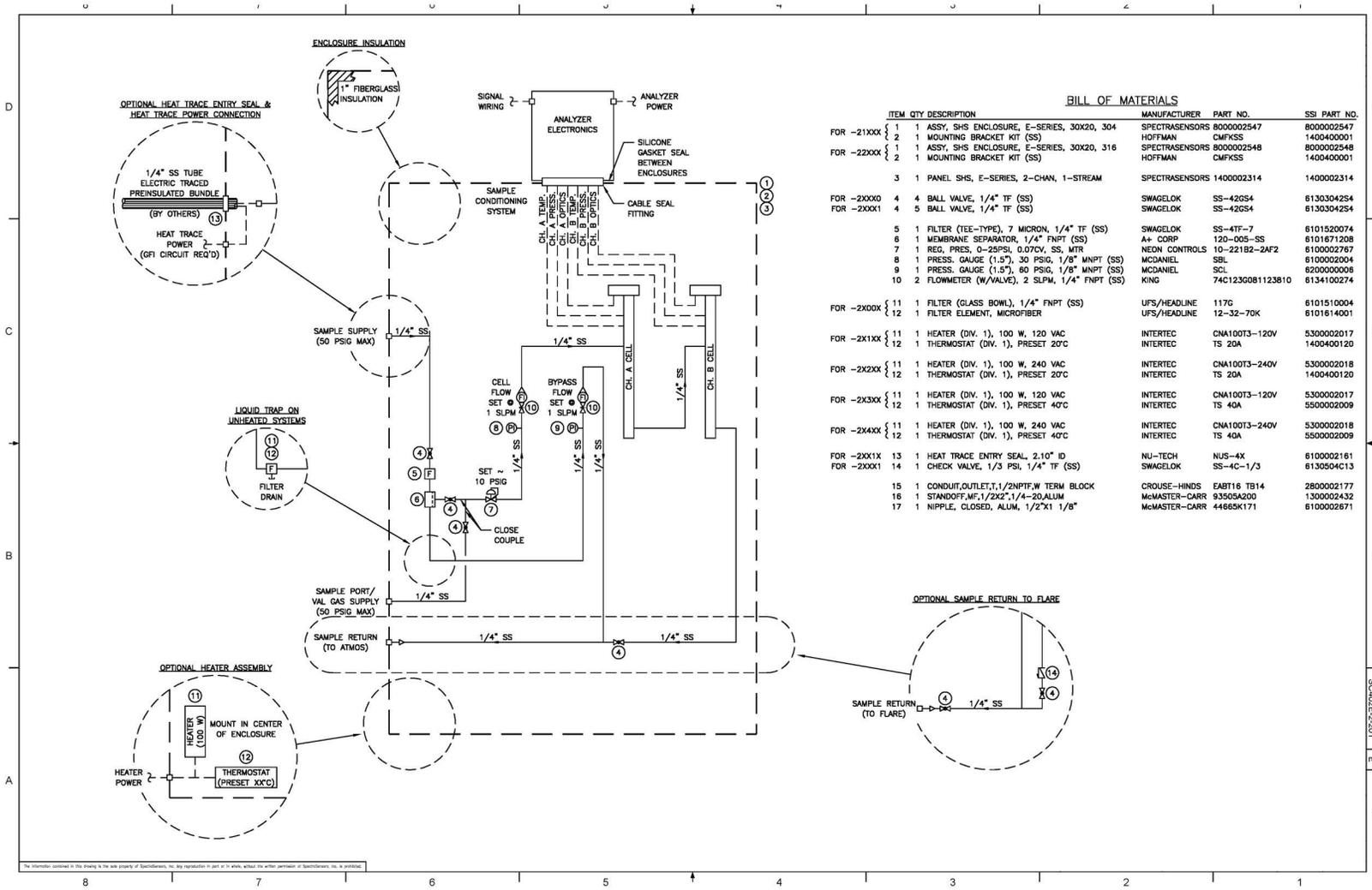
Figure A-5 SS3000e single stream analyzer system sample system schematic
