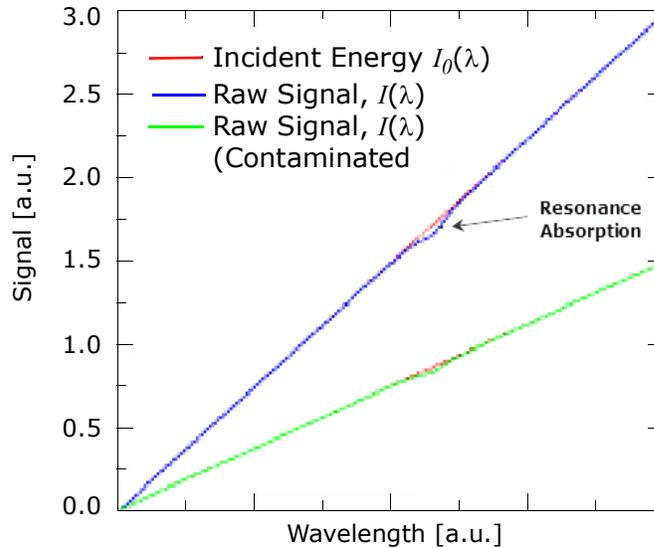
**Figure 1-2** Typical raw signal from a laser diode absorption spectrometer with and without mirror contamination
