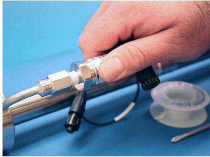
**Figure B-9** Replacing pressure sensor
