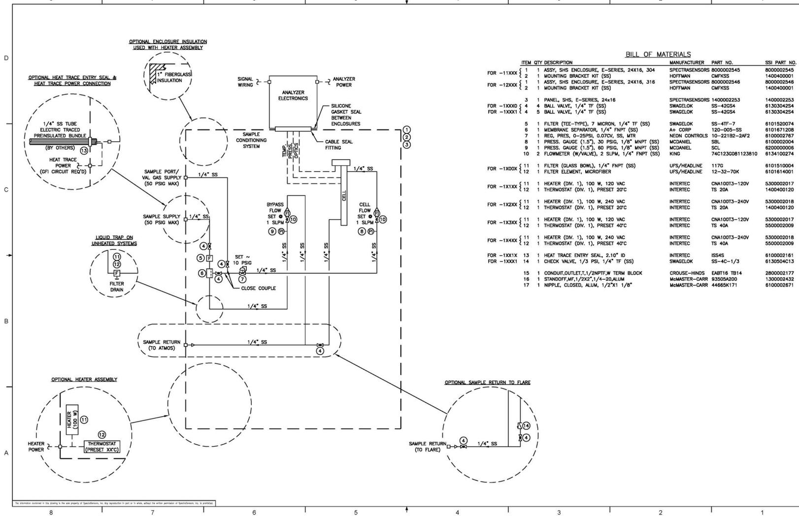
Figure A-2 SS500e/SS2000e analyzer system sample system schematic
