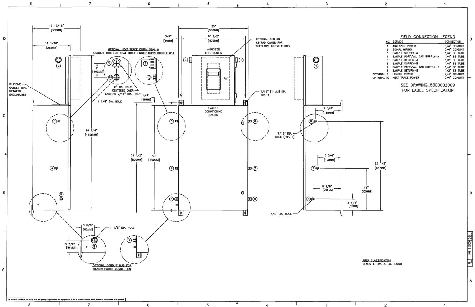
Figure A-7 SS3000e dual stream analyzer system outline and mounting dimensions
