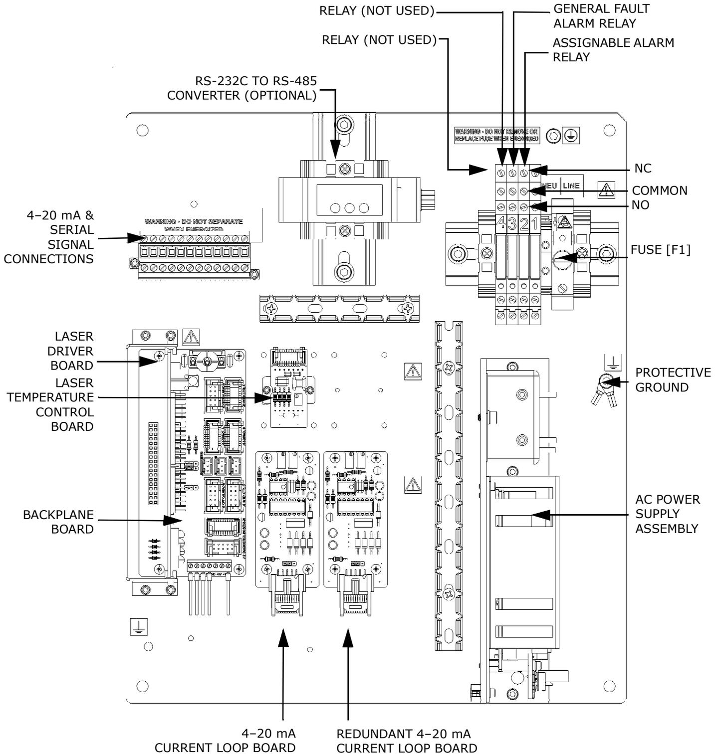
**Figure 1-6** Electronics control board (AC) for single-channel systems (SS500e/SS2000e) with RS-232C to RS-485 converter
