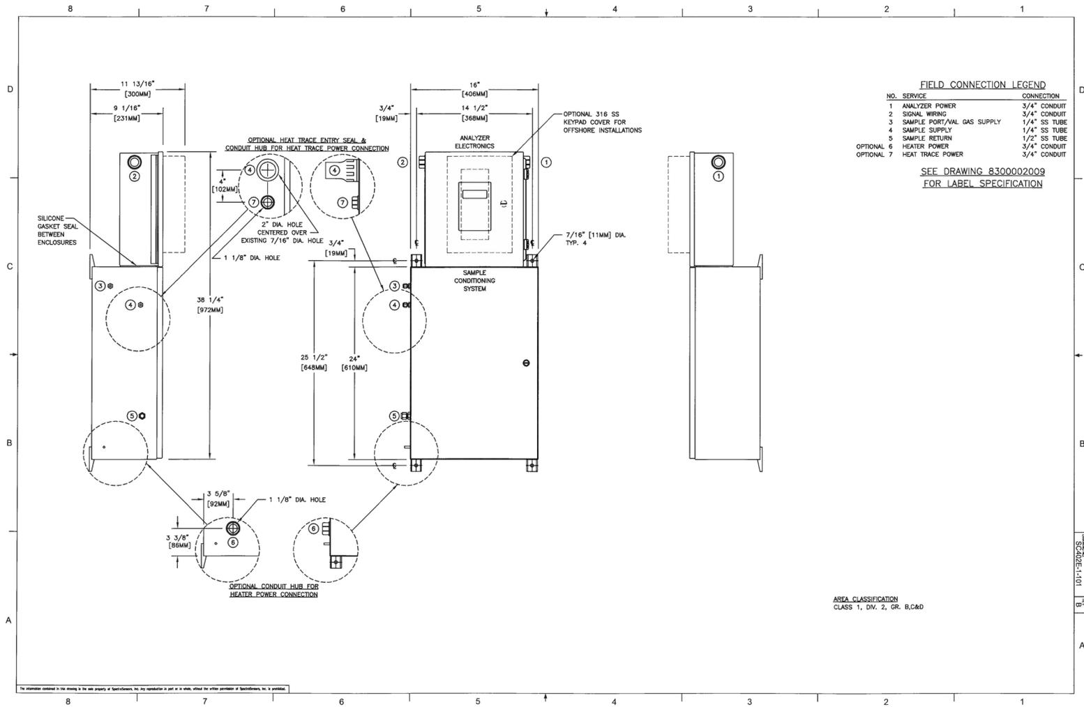
Figure A-1 SS500e/SS2000e analyzer system outline and mounting dimensions
