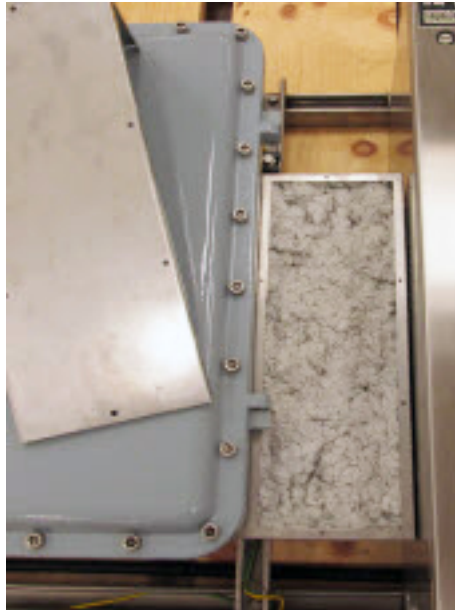
Figure B-19 Unpacking enclosure insulation
