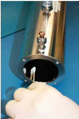
Figure B-8 Removing excess seal tape from inside cell
