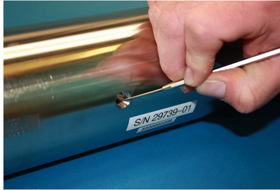
Figure B-7 Removing excess seal tape from flange
