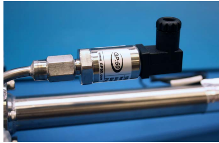
Figure B-17 Newly installed pressure sensor positioning
