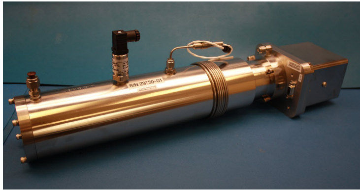
Figure B-11 New pressure sensor installed
