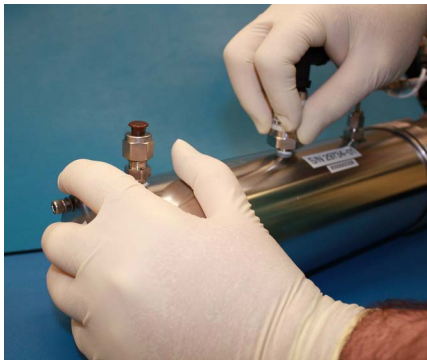
Figure B-10 Replacing pressure sensor
