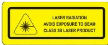
*The sample cell assembly contains a low-power, 20 mW MAX, CW Class 3b invisible laser with a wavelength between 700-3000 nm. Never remove the end mirror unless the power is turned off.*
