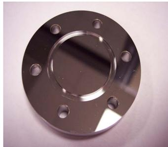
**Figure B-2** *Stainless steel mirror; mirror side up*
