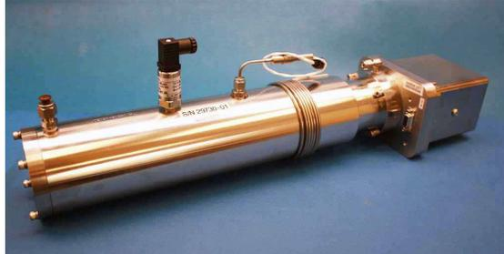
**Figure B-4** Removed measurement cell with pressure transducer face up
