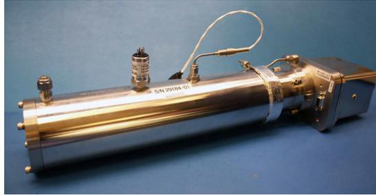
**Figure B-10** New pressure transducer installed
