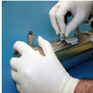
**Figure B-9** Replacing pressure transducer
