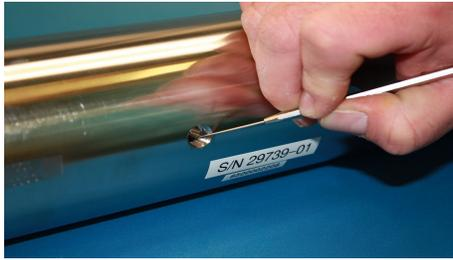
**Figure B-6** Removing excess seal tape from flange
