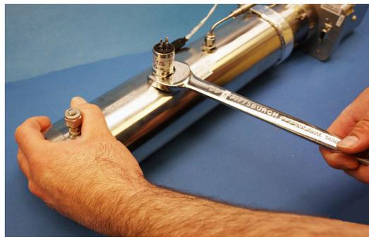
**Figure B-5** Removing the old pressure transducer
