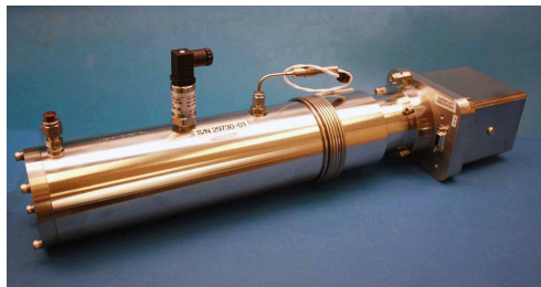
Figure B-4 Removed measurement cell with pressure sensor face up
