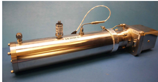
Figure B-10 New pressure sensor installed
