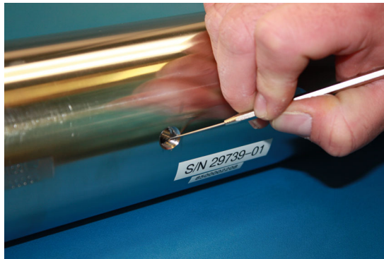
Figure B-6 Removing excess seal tape from flange
