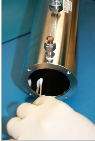
Figure B-7 Removing excess seal tape from inside cell
