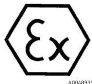
Figure 2. ATEX label for use in hazardous areas
