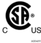
Figure 1. Label showing equipment is approved for use in hazardous areas in the United States and Canada
