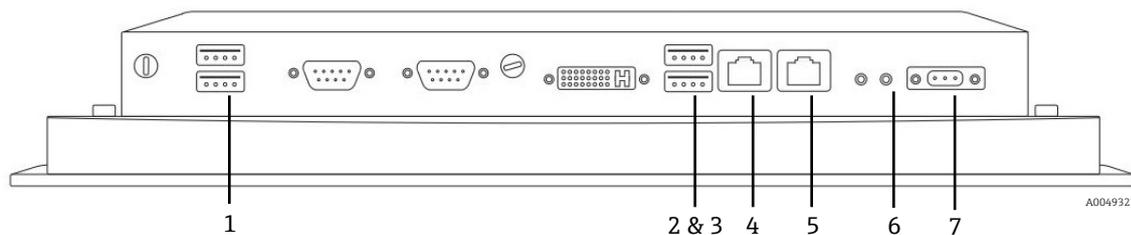
Figure 6. External connections for HMI for use with non-embedded Raman Rxn analyzer and RunTime
