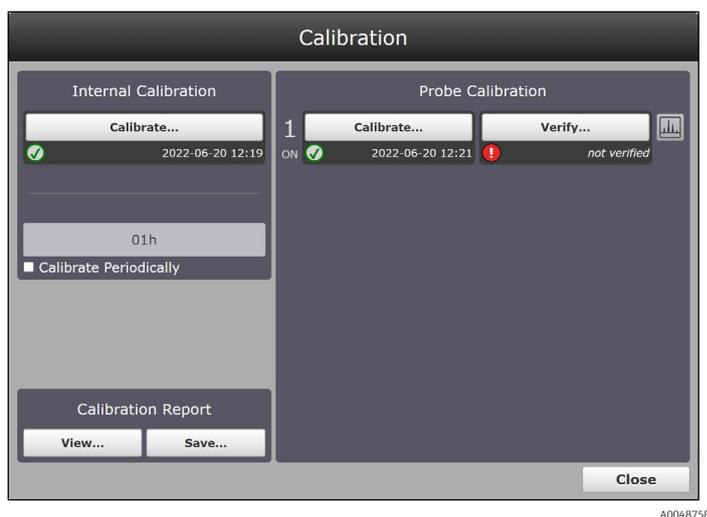
Figure 15. Calibration window with quick view buttons for a Raman Rxn single channel analyzer
