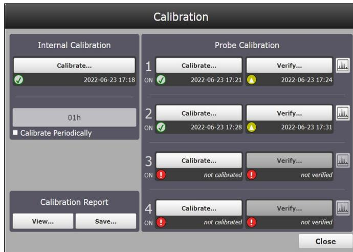
Figure 14. Calibration window with quick view buttons for a Raman Rxn four channel analyzer
