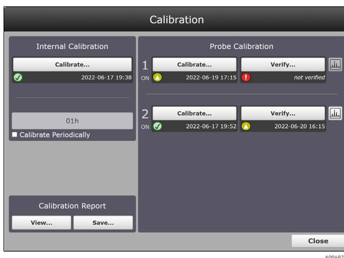
Figure 21. Calibration window for a Raman Rxn Hybrid analyzer
