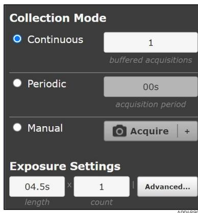
Figure 31. Collection mode details for continuous mode
