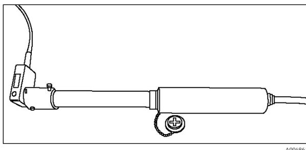
Figure 20. HCA lamp head and extension tube attached to Rxn-20 non-contact optic and probe
