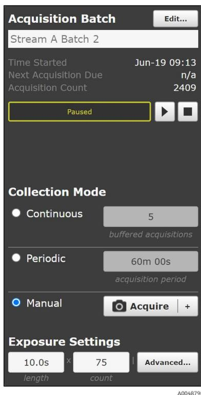
Figure 28. Manual collect mode options
