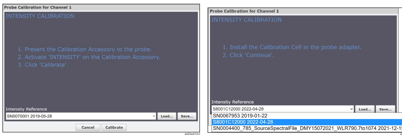
Figure 19. Intensity calibration window in Raman RunTime
