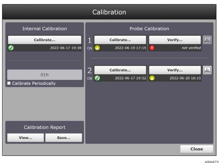
Figure 16. Calibration window with quick view buttons for a Raman Rxn Hybrid analyzer
