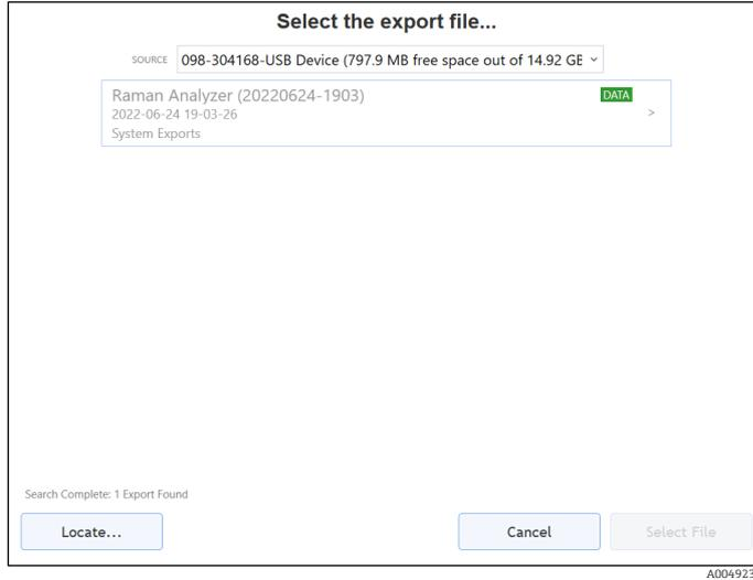
Figure 56. Restoring Raman RunTime to an earlier version using export stored on a USB drive
