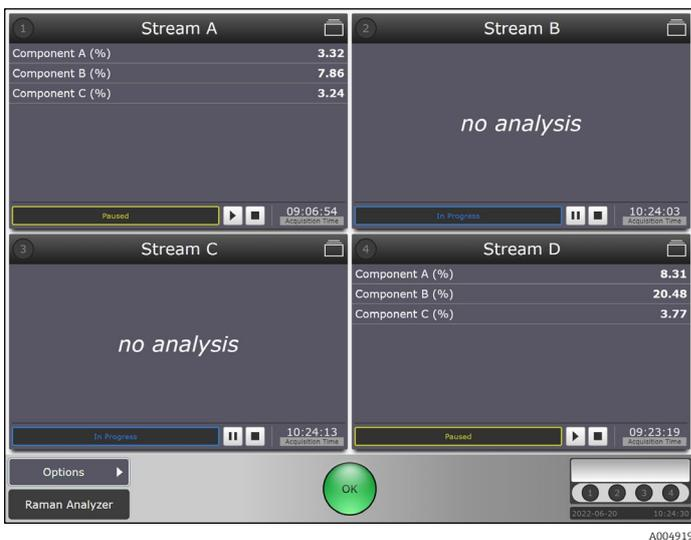
Figure 35. Results for a Rxn2 four channel analyzer with models active for probe 1 and probe 4
