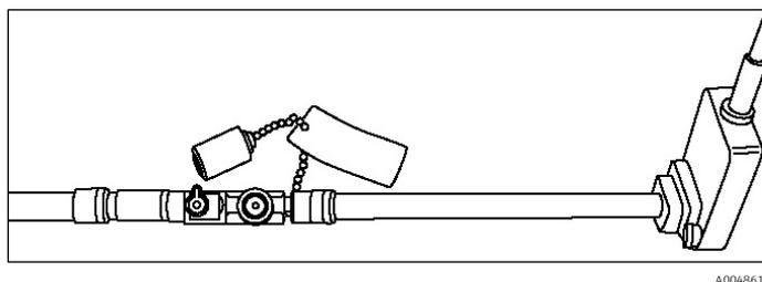
Figure 18. Example of the Rxn-10 probe with a bio-Optic connected to the HCA
