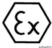
Figure 2. ATEX label for use in hazardous areas
