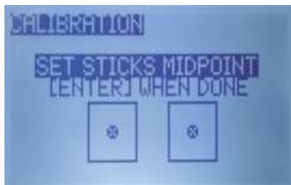
▲ 2. Set the gimbal sticks to the midpoint and press the right button (Enter) for the next step.
