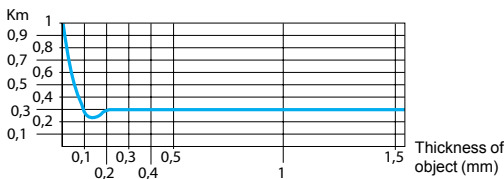
Typical curve for a copper object used with a Ø 18 mm cylindrical sensor
