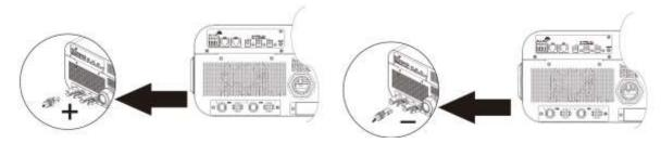
**WARNING!** For safety and efficiency, it's very important to use appropriate cables for PV module connection. To reduce risk of injury, please use the proper cable size as recommended below.
