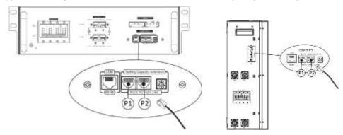
Step 2: Use supplied RJ45 cable (from battery module package) to connect inverter and Lithium battery.
