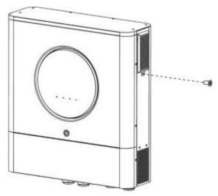
**Step 2:** Then, dustproof case can be removed and take out air filter foam as shown in below chart.
