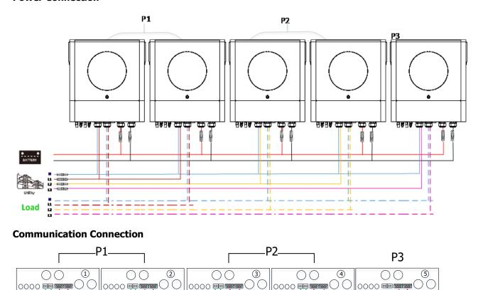
Two inverters in one phase and only one inverter for the remaining phases:
