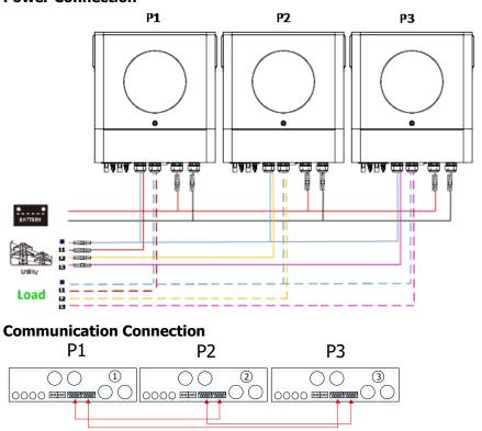
**WARNING:** Do not connect the current sharing cable between the inverters which are in different phases. Otherwise, it may damage the inverters.
