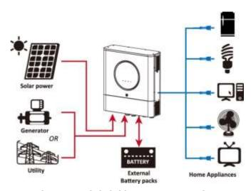
Figure 1 Basic hybrid PV System Overview
