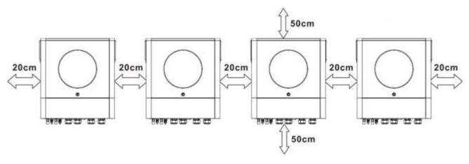
**NOTE:** For proper air circulation to dissipate heat, allow a clearance of approx. 20 cm to the side and approx. 50 cm above and below the unit. Be sure to install each unit in the same level.
