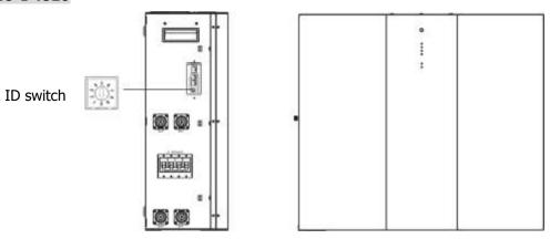
ID Switch indicates the unique ID code for each battery module. It's required to assign a unique ID to each battery module for normal operation. We can set up the ID code for each battery module by rotating the PIN number on the ID switch. From number 0 to 9, the number can be random; no particular order. Maximum 10 battery modules can be operated in parallel.
