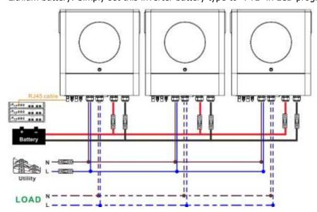
Step 2. Switch on Lithium battery.
