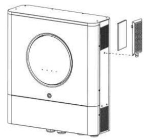
**Step 3:** Clean air filter foam and dustproof case. After clearance, re-assemble the dust-kit back to the inverter.
