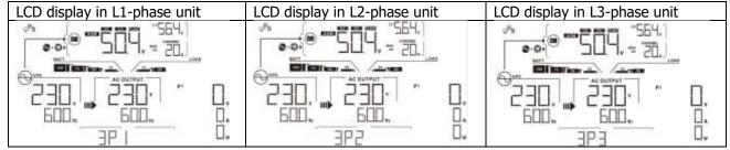
Step 5: If there is no more fault alarm, the system to support 3-phase equipment is completely installed.
