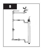
Close the downstream tap once the UV chamber is filled with water, and inspect for any leakages.
