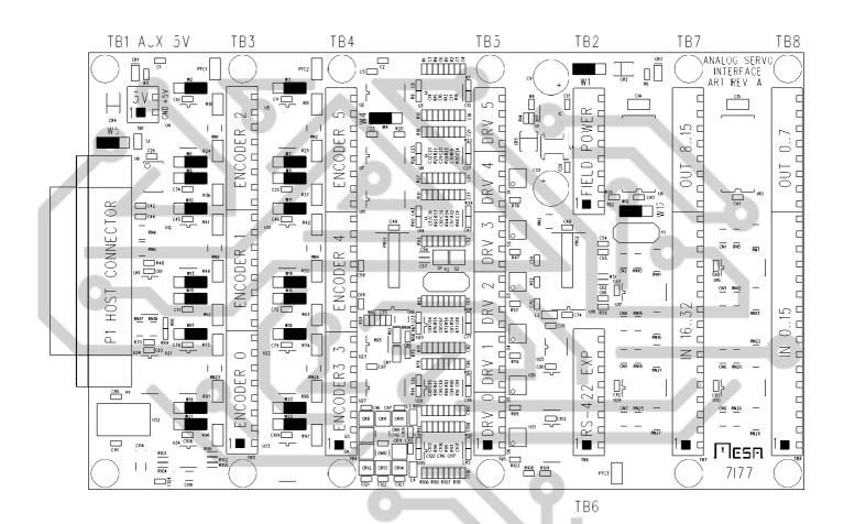
Note: Terminal block pin 1s are marked with a square
