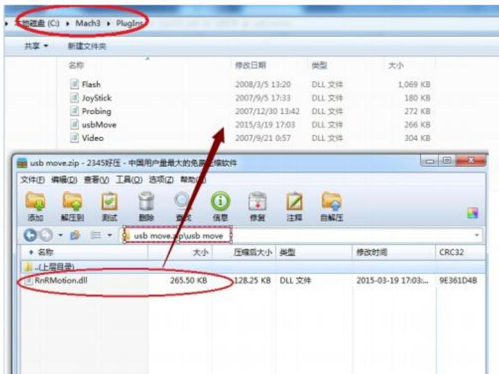
1.3.3 Start the Mach3software, a dialogue of “Motion Control Hardware PlugIn sensed!” is shown. Please select the“RnRMotionControllerECO-V2.0”,you can also check”Don't ask me this again”
