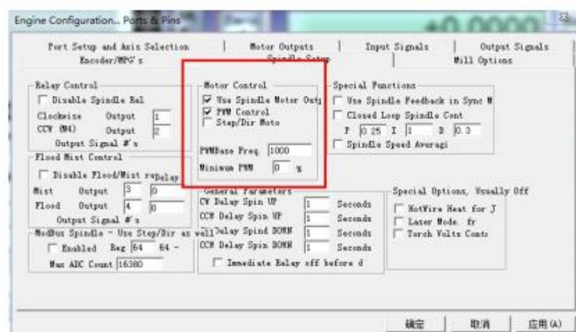
Enable spindle output. as shown below:
