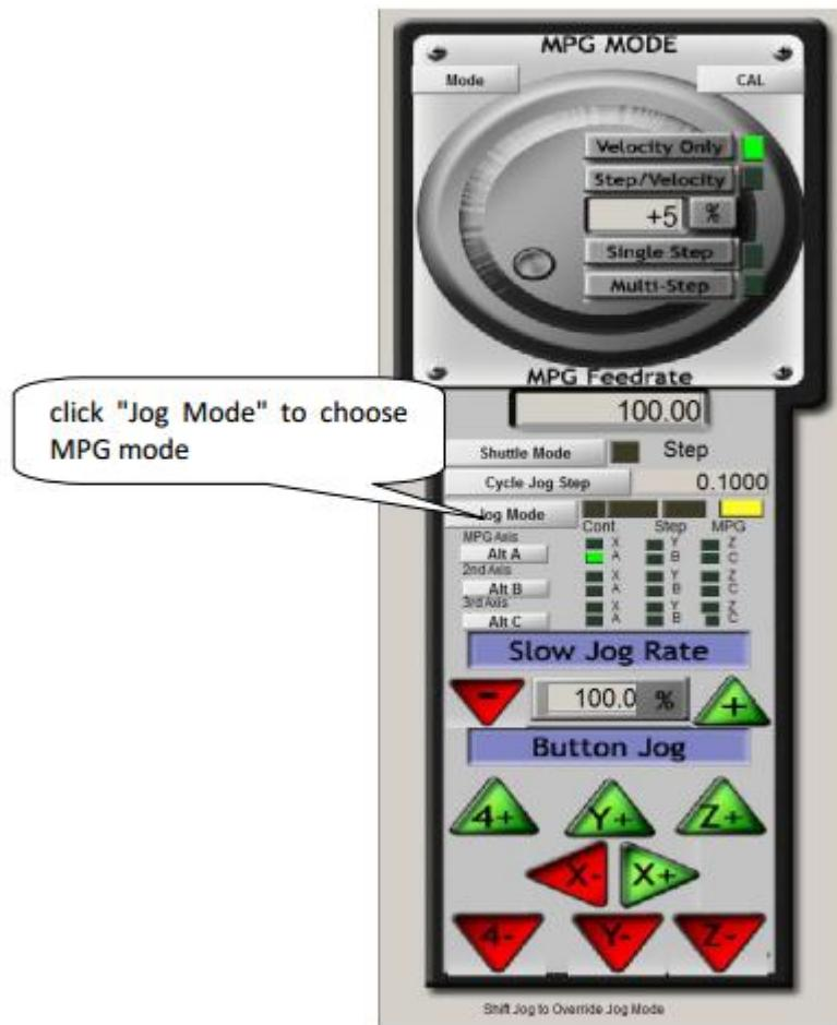
Click the "Jog mode" select MPG mode, you can use the electronic handwheel control the motor
