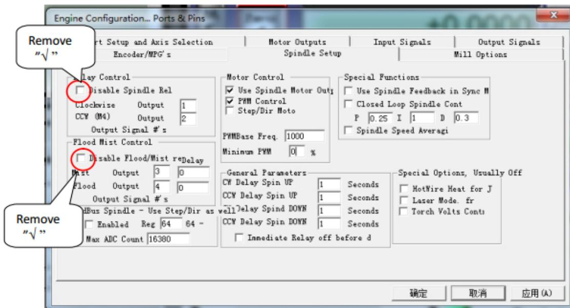
M3 code control output 1 output,M4 code control output port 2 output,M5 shut down output1 and output2.
