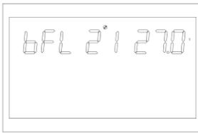
Figure 1-31 Floating charge mode voltage point setting page
