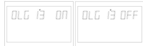
Figure 1-23 Overload convert to bypass setting page
