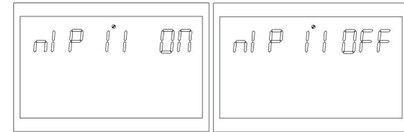
Figure 1-21 Main input power failure alarm setting page
