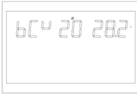
Figure 1-30 Constant voltage mode voltage point setting page
