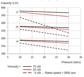
Data shown take into account a wear margin. Do not oversize the pump when selecting the gear capacity.
