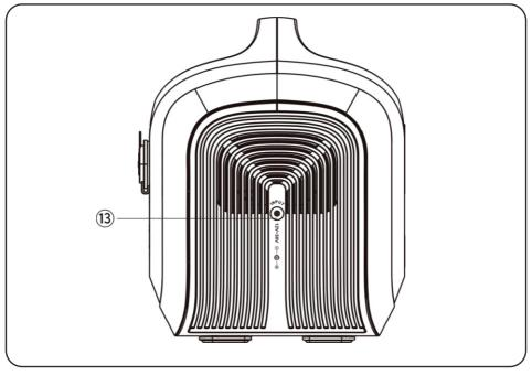
1.AC Output Port 2.AC Output Power On/Off Switch 3.Main Power On/Off Switch 4.Car Charger and DC5521 Output Ports Power On/Off Switch 5.12V Car Charger Output Port 6.12V DC5521 Output Port 7.USB-C Input & Output Port 8.USB-A Output Port 9.USB-C & USB-A Output Power On/Off Switch 10.LCD Screen 11.LED Light Power On/Off Switch 12. LED Light 13.7909 Recharging Input Port
