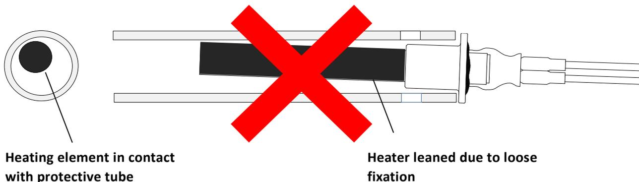
Please make sure to let an interspace of minimum 3mm around the ceramic heating element and the tube.
