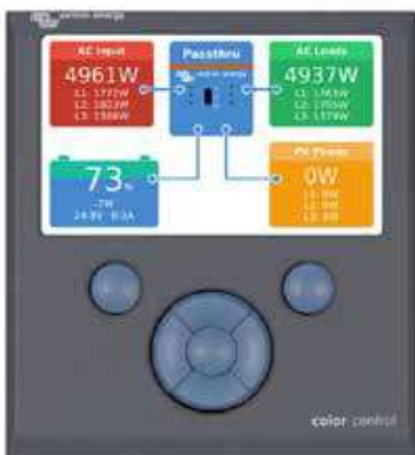
Color Control GX, showing a PV application
