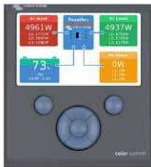
Color Control GX, showing a PV application
