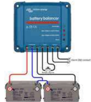
Battery Balancer (BMS012201000) The Battery Balancer equalizes the state of charge of two series connected 12V batteries, or of several parallel strings of series connected batteries. When the charge voltage of a 24V battery system increases to more than 27V, the Battery Balancer will turn on and compare the voltage over the two series connected batteries. The Battery Balancer will draw a current of up to 1A from the battery (or parallel connected batteries) with the highest voltage. The resulting charge current differential will ensure that all batteries will converge to the same state of charge.
