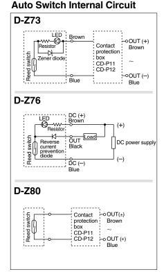
Note 1) Operating load is an induction load. Note 2) Wiring to the load is 5 m or longer. Note 3) Load voltage is 100 VAC. Use the contact protection box in any of the above listed situations. The contact point life
