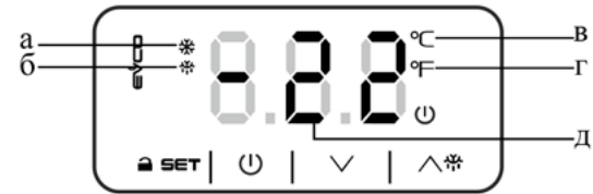
Pic.7 Electronic controller EVCO
