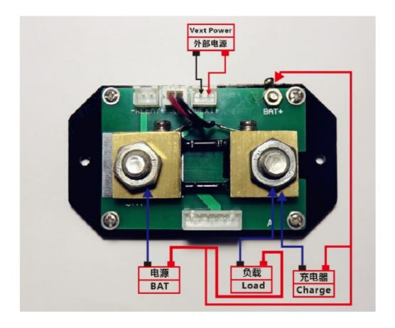
explanation:If the voltage range of the tested battery (power supply) during normal operation is not between (6-75V), the external power supply connection mode can be used external supply voltage range (6-75)V,First adjust the jumper cap that selects the power supply interface to "3W",then connect the positive terminal of the battery (power supply) to the voltage
