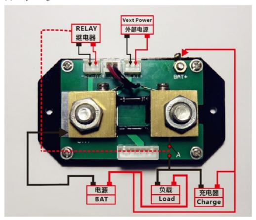
explanation: the operating voltage of the relay is provided by an external power supply if the relay is configured, an external power supply with the
